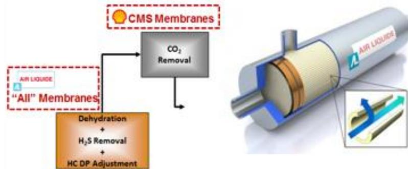
Carbon Molecular Sieve (CMS) Membranes: more efficient membranes for CO<sub>2</sub> separation from natural gas
