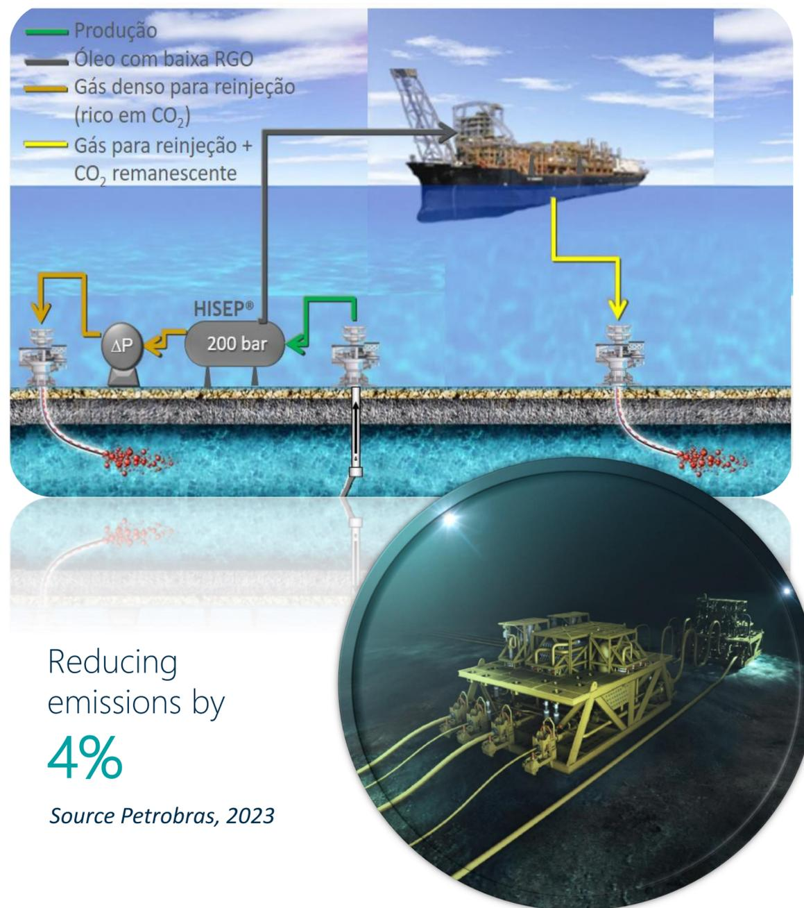
The high pressure **CO<sub>2</sub> separation technology (HISEP)** is a solution that allows the gas leaving the reservoir to be separated and reinjected from a system located on the seabed.
