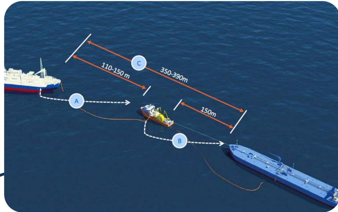
The CTV (cargo transfer vessel) technology is a cost efficient, flexible, safe and energy saving method of transferring oil from offshore oil fields onto conventional tankers.
